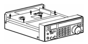
**3** Pull the PCB towards the front panel and lift it as shown in the diagram.
