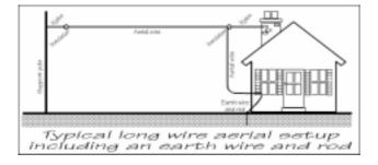
Keeping the aerial away from supports and building will reduce the loss of signal from the wire aerial and prevent unwanted noise from entering the aerial system.
