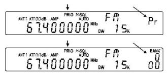
Use the *MAIN DIAL*, *SUB DIAL* or enter a three digit memory location via the numeric keypad. To transfer the data to PRIORITY press [ENTER].
