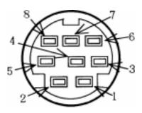
A standard 8-pin mini-din connector is used (which is widely available or the optional CR5000 tape lead may be used). The pin-outs for **ACC 1** are as follows:
