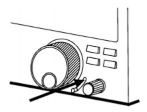
**2** Using a match stick or similar *tool*, press and release the reset switch (with the AR5000 switched on and powered in the normal manner).
