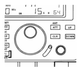
A tuning knob is by far the most *traditional* approach to tuning on short wave, the *MAIN DIAL* provides a smooth feel and the best method of user interface especially when listening on the SSB, FAX and CW modes. The *SUB DIAL* is indented so tunes in a number of clicks and is best suited for channelised tuning on the VHF/UHF bands.
