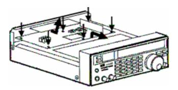
**4** Locate position **MF1** on the I.F. PCB (refer to illustration). The position is currently unoccupied ready for the optional 500 Hz Collins mechanical filter. Use a desoldering pump to remove any excess solder from the respective pin positions. Insert the CW filter into the cleared holes of the PCB and securely solder its pins - don't overheat the filter!
